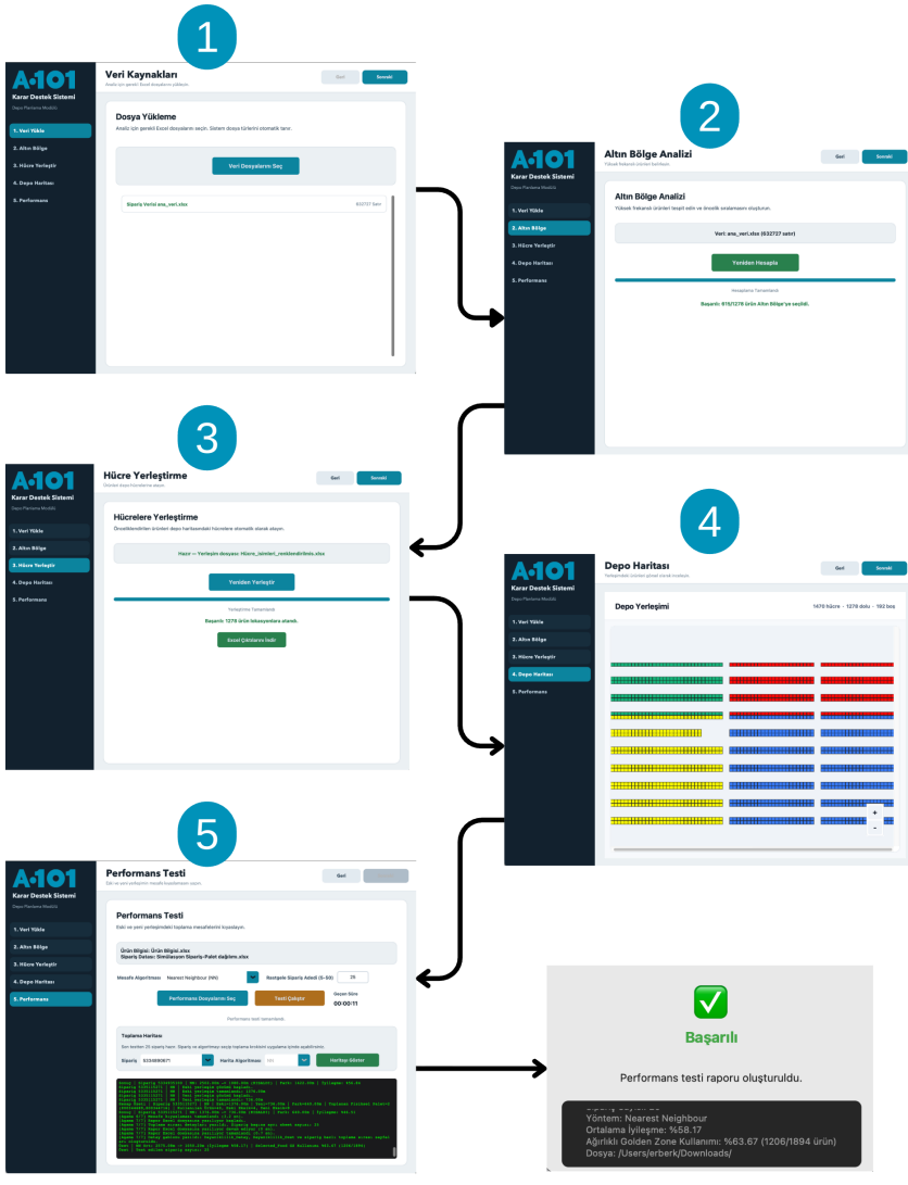
Figure 12.7: DSS five-step workflow: data upload (Step 1), Golden Zone analysis (Step 2), slotting (Step 3), map visualization (Step 4), and performance testing (Step 5).
